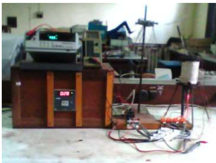
Figure 3 Photograph of the experimental setup of electrical resistance and capacitance measurement
