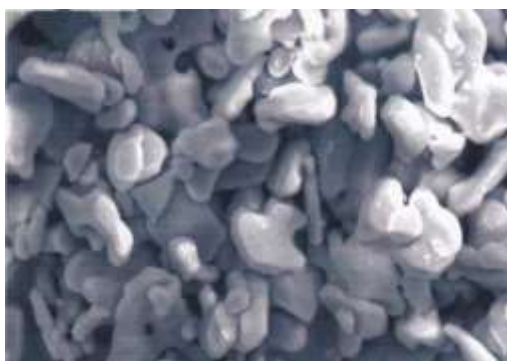
Figure 3. SEM photograph of Al 2 O 3 powder
