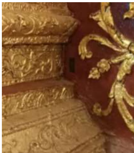
Figure 3(a). CR-39 detector S1 under the Buddha Image
