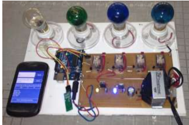
Figure 7: The photograph of four channel Bluetooth control system
