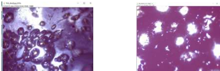
Figure 5. Optical Micrograph of pure PVA and SCRF reinforced PVA Films
